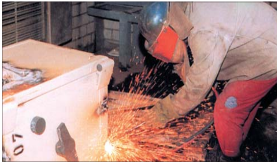
Fig. Test method with cutting torch (above) and with diamond core drill (right)
