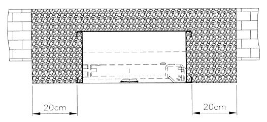
Wall safes are top heavy. The opening of a not built-in wall safe causes danger of tipping over.
