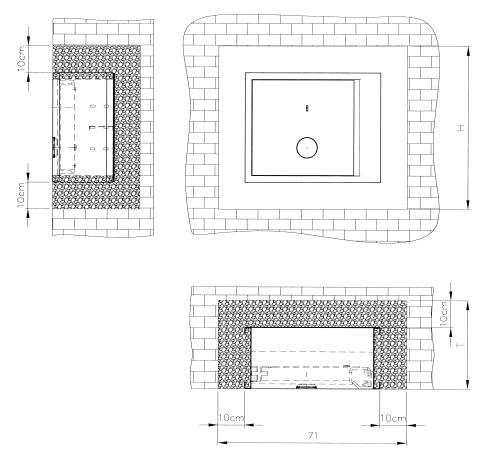
2.2.1 For the installation of a wall safe without rear wall armor a minimum wall opening according to the following table has to be prepared:
