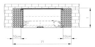
2.1.1 For the installation of a wall safe with rear wall armor a minimum wall opening according to the following table has to be prepared:
